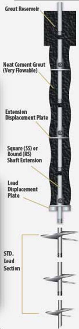
Screw Pile Section
